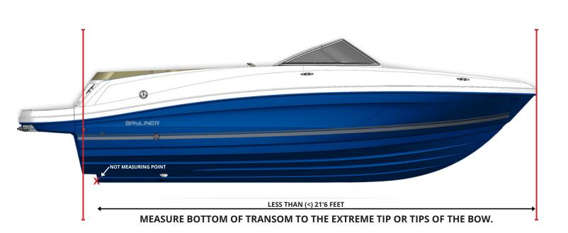
Boats pictured below are for measurement reference only. These are examples, not rules. Lake & Marina Section 7.2a (Guidelines For Measuring Non-Pontoon Boats) and Section 7.2b (Guidelines For Measuring Pontoon Boats) in the Canyon Lake POA's Rules & Regulations provide specific rules for boat measurements. Boat photos are style examples only and not representative of any make or model being acceptable or not.
