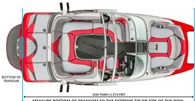
MEASURE BOTTOM OF TRANSOM TO THE EXTREME TIP OR TIPS OF THE BOW. PICKLEFORKS ARE **NOT** MEASURED AT THE CENTERLINE.
