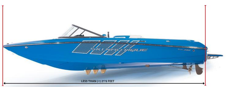
MEASURE BOTTOM OF TRANSOM TO THE EXTREME TIP OR TIPS OF THE BOW. V-NOSE BOATS ONLY. PICKLEFORK SHAPED BOATS ARE MEASURED TO THE EXTREME TIPS OF BOW.
