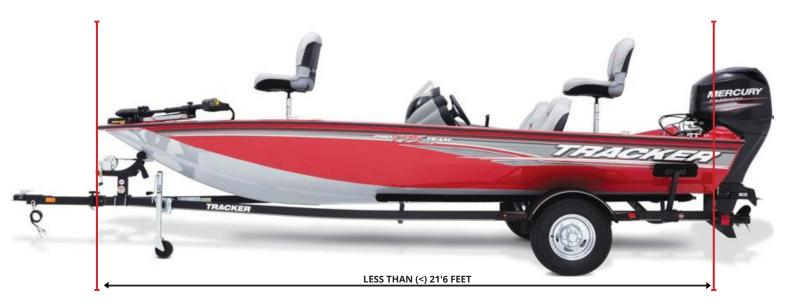
MEASURE BOTTOM OF TRANSOM TO THE EXTREME TIP OR TIPS OF THE BOW AT CENTERLINE.
