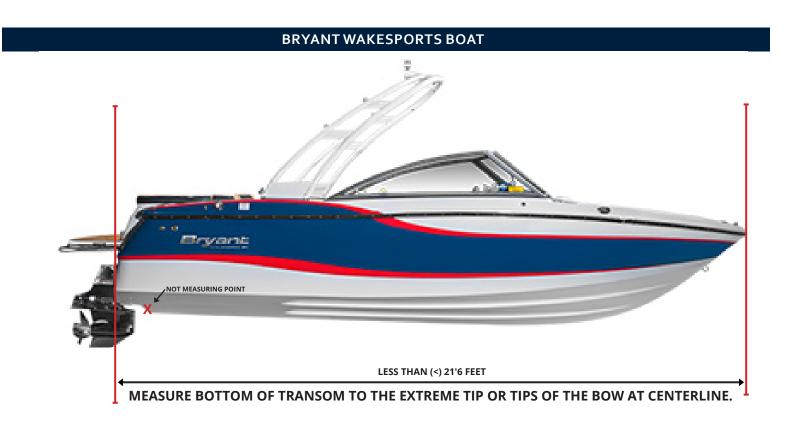
Boats pictured below are for measurement reference only. These are examples, not rules. Lake & Marina Section 7.2a (Guidelines For Measuring Non-Pontoon Boats) and Section 7.2b (Guidelines For Measuring Pontoon Boats) in the Canyon Lake POA's Rules & Regulations provide specific rules for boat measurements. Boat photos are style examples only and not representative of any make or model being acceptable or not.
