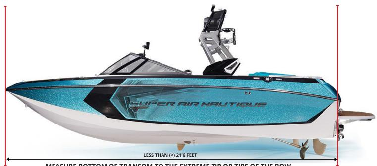
MEASURE BOTTOM OF TRANSOM TO THE EXTREME TIP OR TIPS OF THE BOW. V-NOSE BOATS ONLY. PICKLEFORK SHAPED BOATS ARE MEASURED TO THE EXTREME TIPS OF BOW.
